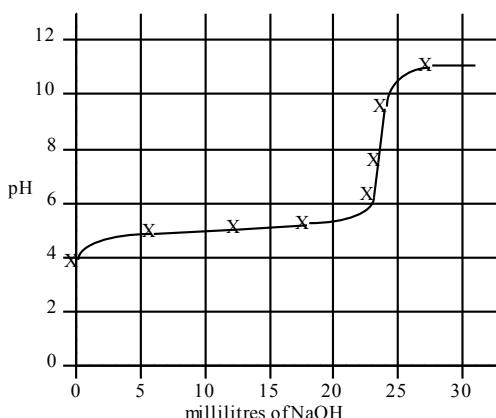
A 30.00 millilitre sample of a weak monoprotic acid was titrated with a standardized solution of NaOH. A pH meter was used to measure the pH after each increment of NaOH was added, and the curve above was constructed.
